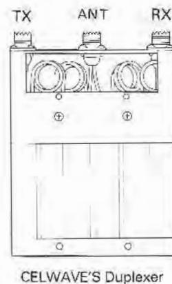
**Note :** When making adjustments after installing the duplexer, remove the front panel and hold down the sub-panel (21), then perform adjustments from the adjusting holes (22).
