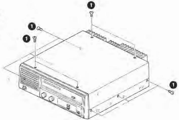
2. Remove the 11 screws ( ❷ ) retaining the shield cover to remove the shield cover.
