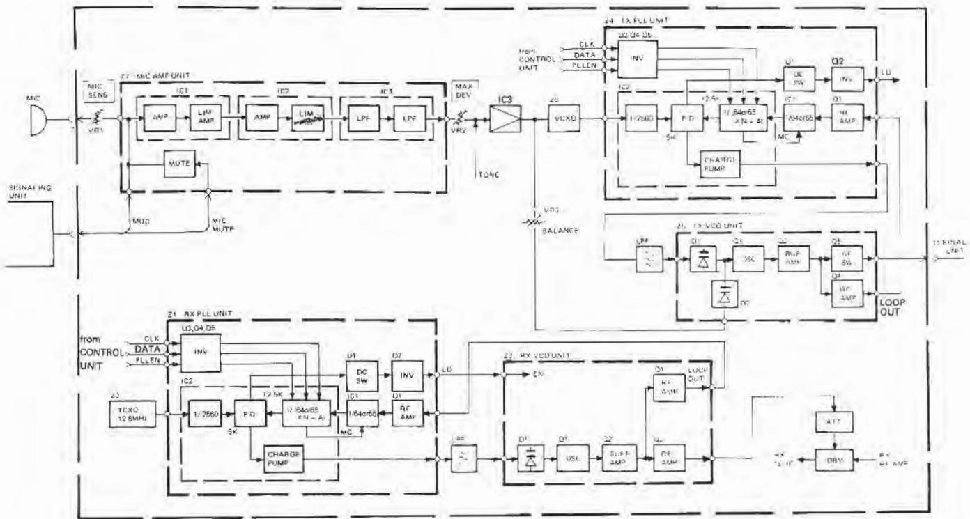
Fig. 4 PLL & Modulation circuit block diagram
