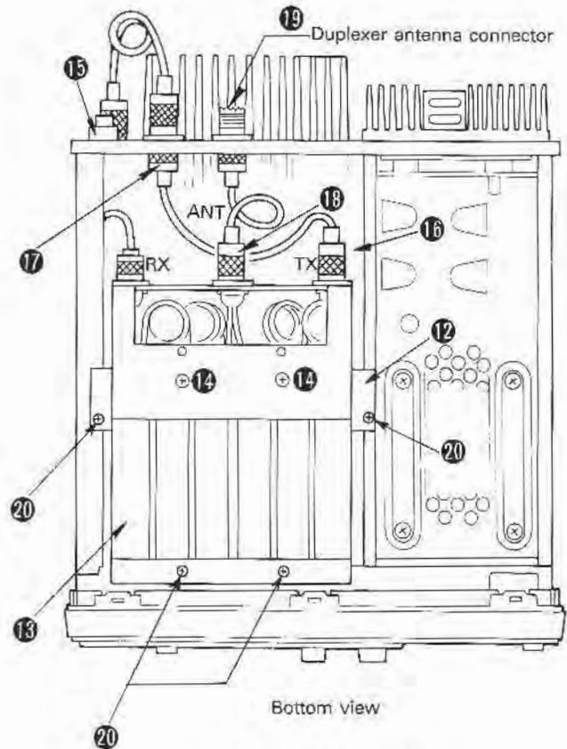
**Note :** The input/output connectors of the duplexer manufacture by CELWAVE are located as shown in the figure. Pay attention when connecting the connectors.
